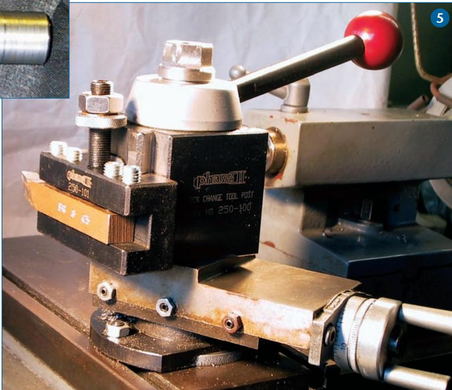
the bottom plate on the quick-change post was just a “taste” smaller than the ID of the central cylinder. I had to reduce the last 1/2” of the adaptor diameter so it would slide all the way through. The last operation is to saw ff the blank above the hex top and you’re done! *Photo 4* shows the completed adaptor and *Photo 5* shows the new quick-change post mounted on the 9” × 20” lathe and ready to go!
